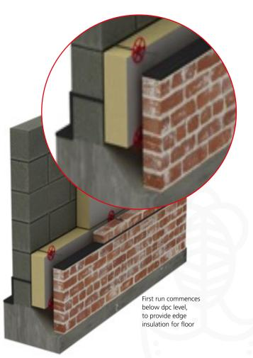
Figure 1 - Insulation installed below dpc level to provide edge insulation for floor.
